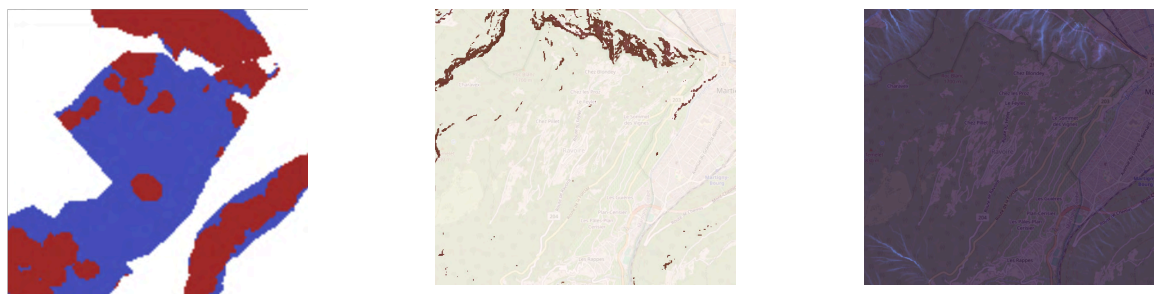
Figure 15 - Problematic area, showing the predicted hazard map for the Heuristic + Grid Search model (left), the source cells (middle) and the RockyFor3D trajectories (right).
