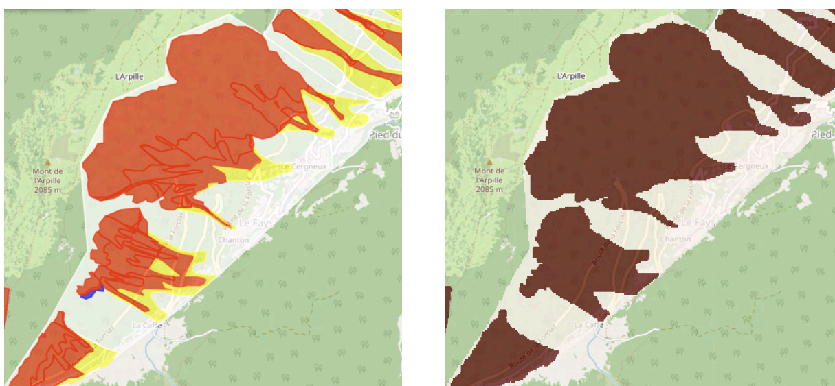
Figure 9 - Comparison of the hazard zones as vector polygons (left), and as converted raster cells (right). The rasterized hazard zone is binarized, with cells of any hazard level being considered as positive samples (red), and cells with no hazard being considered as negative samples (white).
