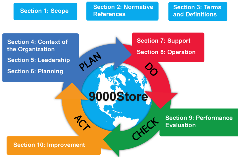
Figure 1 - ISO 9001 requirements on the Deming Wheel (Standard Store 2022)
