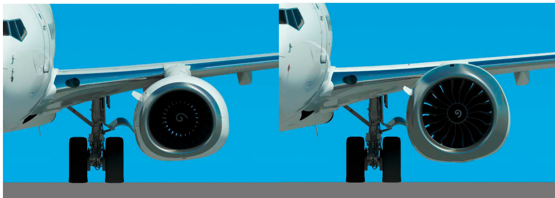
Figure 3 - 737 NG (left) vs 737 MAX (right)
