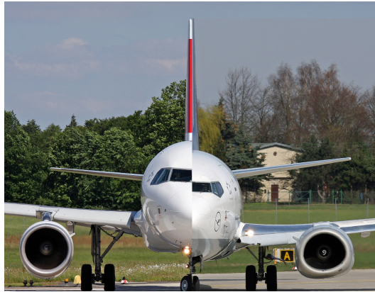
Figure 2 - A320 NEO (left) vs 737 MAX (right)
