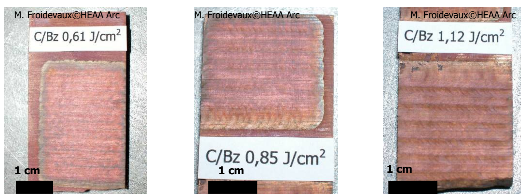
Figure 66 - 67 - 68 Photos of laser cleaned cuprite on bronze at each fluence level 0.61 (left) and 0.85 J/cm 2 (centre) and 1.12 J/cm 2 (right), showing a very low discoloration level to grey.
