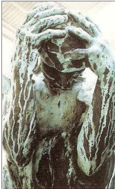
Figure 5 Corrosion details on the figures of Les Bourgeois de Calais from Rodin. The black deposits are visible in the areas sheltered from rain and the black and green streaks due to the flowing rainwater (From Amarger, 2001, p.215).
