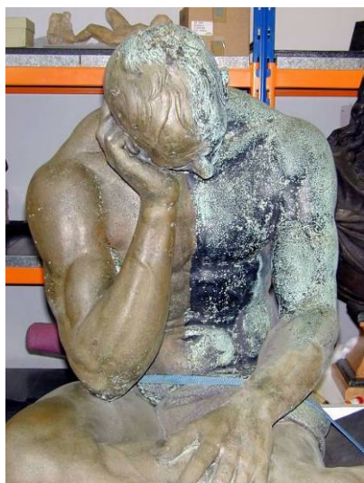
Figure 20 - 21 A half-laser cleaned prisoner.
