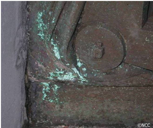
Figure 11 Left: Active corrosion on a bas-relief.
