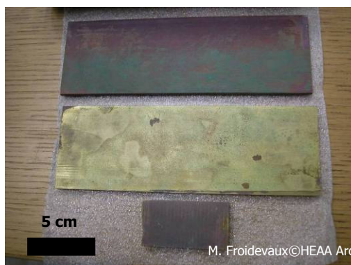
Figure 46 Bronze plates after the first two weeks in brochantite solution.
