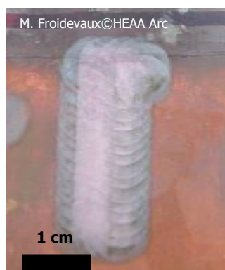
Figure 45 Laser cleaning test on a cuprite copper sample at low fluence (0.44J/cm 2 ).
