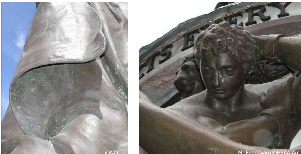
Figure 28 Active corrosion on the drapery of Queen Victoria - June 2006.
