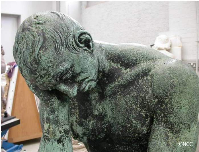
Figure 9 Left: View on a prisoner. One sees clearly the black paint appearing through the green corrosion products.
