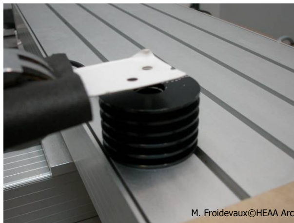
Figure 56 (right) Template positioned on the detector for energy measurements.
