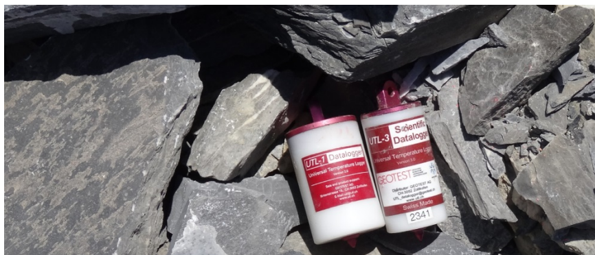
Fig. 3.2: UTL-1 and UTL-2 miniature data loggers measuring GST in the field.
